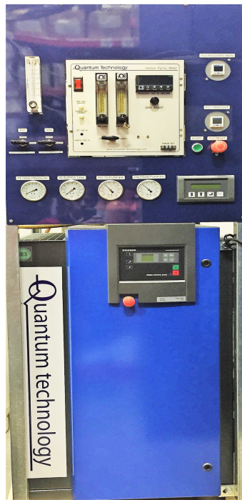
Helium detector integrated in HR3 recovery compressor
